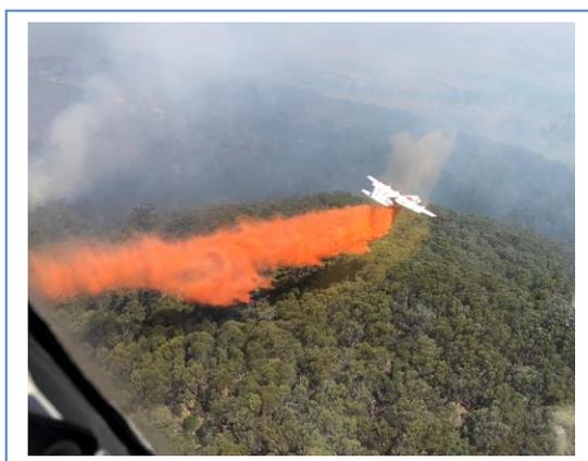
The second photo shows a Hercules fire bomber dropping fire retardant chemicals on to a fire. Peter's job as an Air Attack supervisor is to ensure the retardant is put in the right place in an effective, efficient and safe manner. Following a job like this the group always gets together to discuss what was done right, what was done not as well as it could have been. When you document lessons learnt, it leads to improvements being made.
